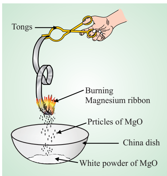
Fig. 4.1: Burning of magnesium ribbon
