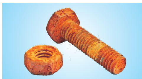
Fig. 4.9: Rusted nuts and bolts of iron
