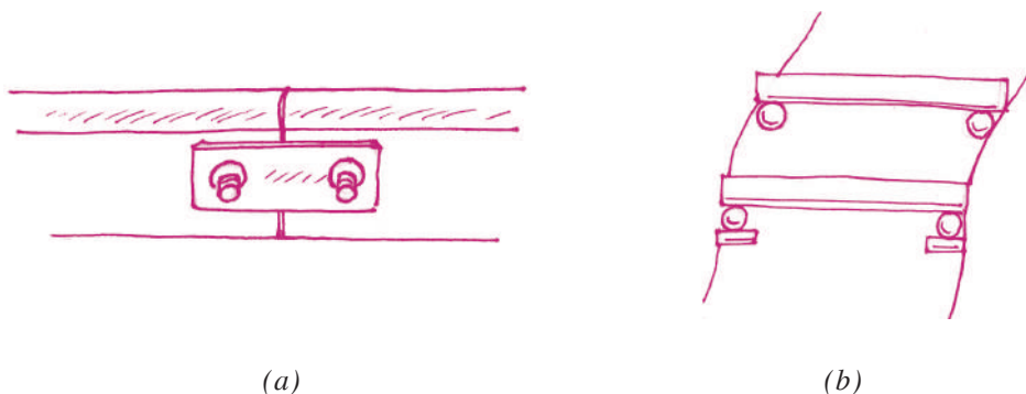
Fig. 14.12 (a) Gap in railway tracks (b) Girders in iron bridges placed on rollers
